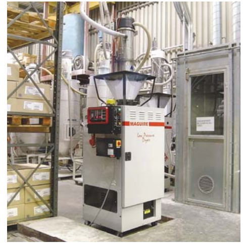
LPD™ dryer tested at Automotive Lighting UK showed potential for substantial cost savings over conventional dehumidifying dryer.
