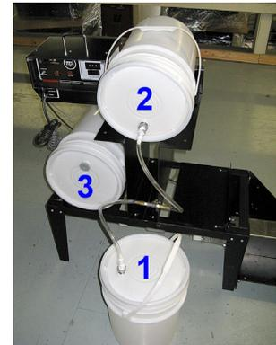
**Step 3** - To change out the empty pail, place the empty pail on the floor and remove the quick disconnect fitting.
