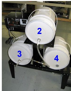
**Step 5** - Place pail #3 on the lower tier. When the top pail color is low, repeat the process from step 2.
