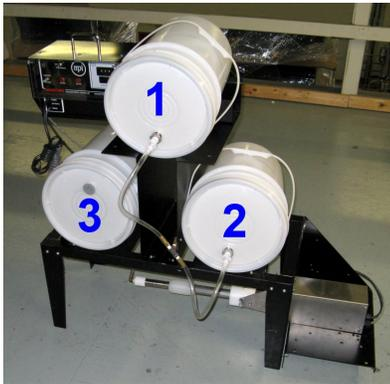
**Step 1** - The main supply pail (1) should be placed at the top of the stand and connected to the supply line. The secondary pail (2) should also be connected to the supply line.
