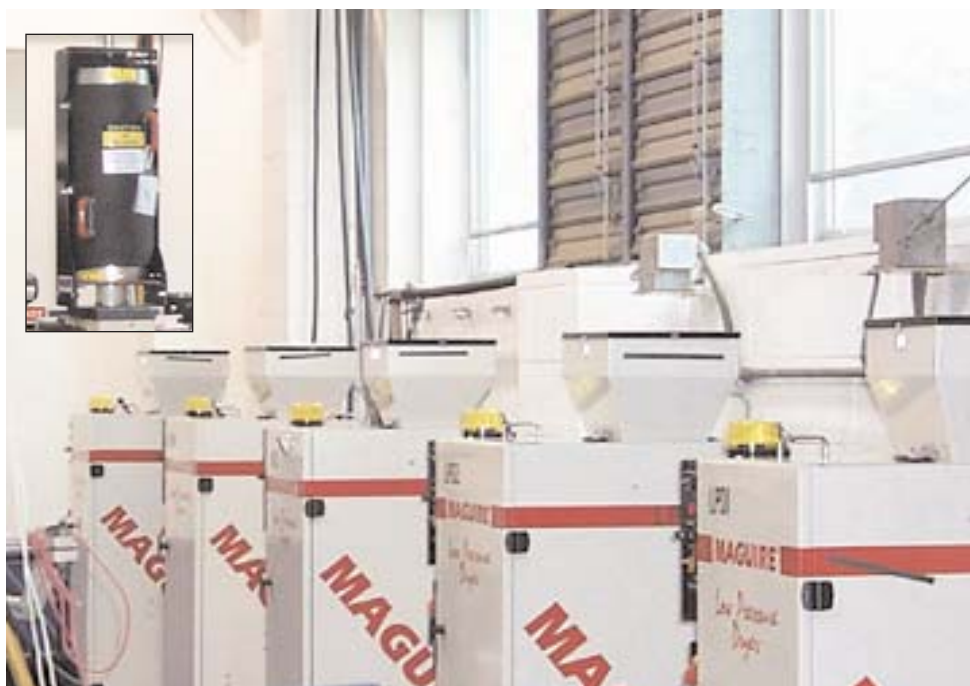
Five LPD-30 dryers in LNP lab increased productivity dramatically. Inset shows canister with dried resin, mounted atop molding machine after removal from dryer.
