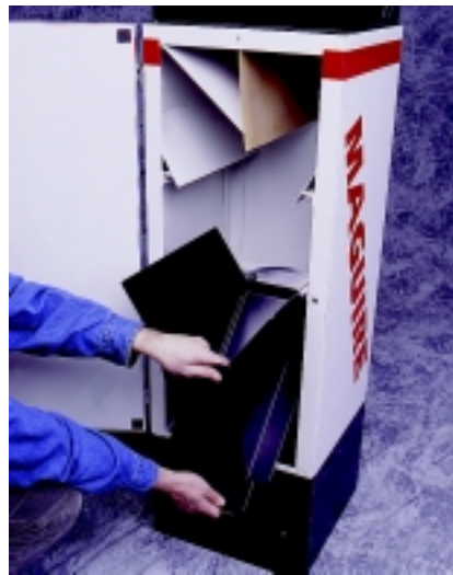
Inner hopper removal
