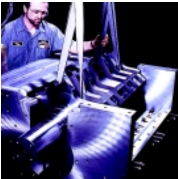
Easy rotor removal through top of cutting chamber
