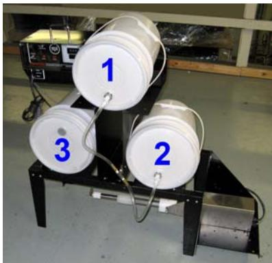
**Step 1** - The main supply pail (1) should be placed at the top of the stand and connected to the supply line. The secondary pail (2) should also be connected to the supply line.
