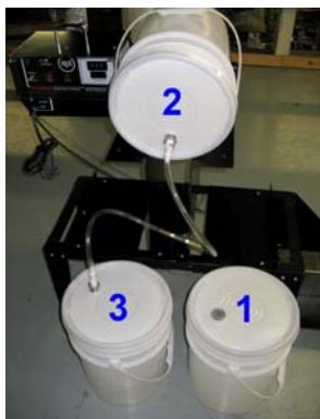
**Step 4** - Place pail #3 on the floor and attach the supply line.
