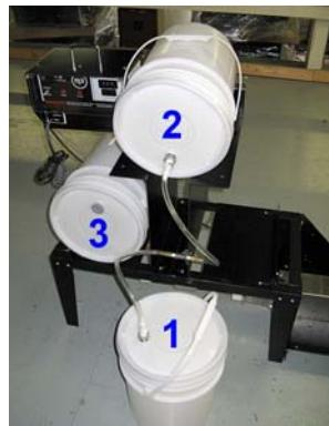
**Step 3** - To change out the empty pail, place the empty pail on the floor and remove the quick disconnect fitting.
