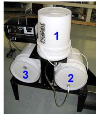
**Step 2** - When the main pail is low, tilt upward on the lid to extract as much color as possible. As the main pail depletes (1), color is extracted from the secondary pail (2).
