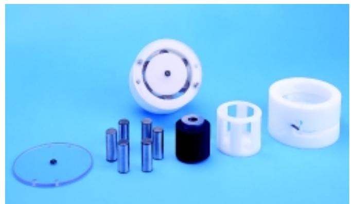
Because tube compression is determined by the depth of this groove, tolerances will not change over time, and priming and pumping accuracy is never lost. In this patented design there are no bearings. The rolling dowel pins do not wear out. A clear viewing window allows observation of the roller and tubing.
