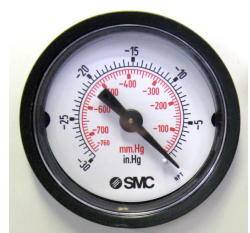
Example of an analog differential pressure sensor gauge. (SMC part# 4300751)
