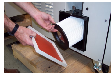
LPD 100, 200 filter location (left side of Dryer)
