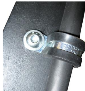
P-clips to secure wire
