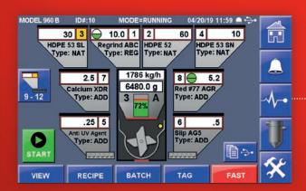
**FlexBus Lite** is integrated with our touchscreen controller for loading multiple materials into a blender.
