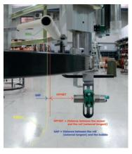
**Gap Sensors** To maintain distance between cage and bubble using ultrasonic signals.
