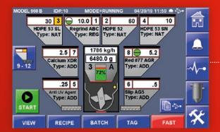
**FlexBus Lite** is integrated with our touchscreen controller for loading multiple materials into a blender.
