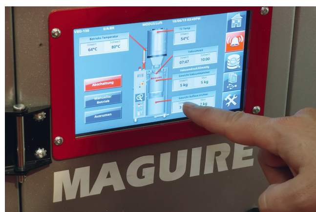
▲ A simple touchscreen is used for the vacuum dryer settings. Important process information, such as output and energy consumption, is available at any time.
