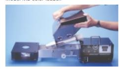
MCF Hopper being removed
