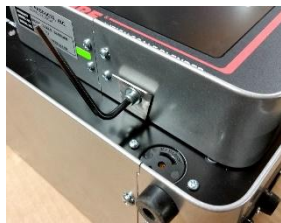
Remove Allen bolt from base of controller.
